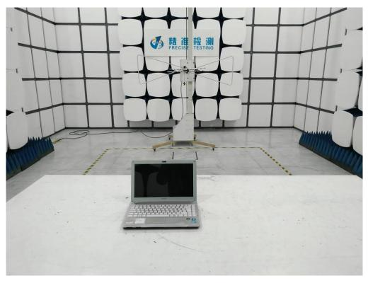
RADIATED EMISSION TEST SETUP ABOVE 1GHz
