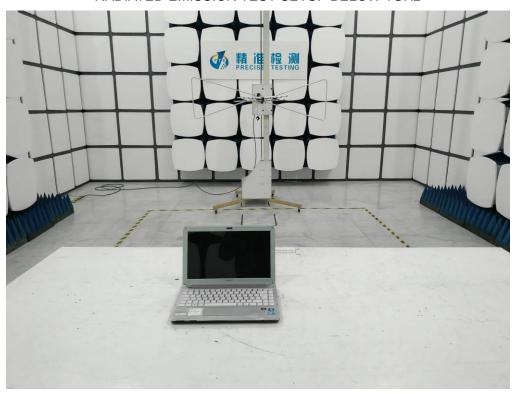
RADIATED EMISSION TEST SETUP ABOVE 1GHz
