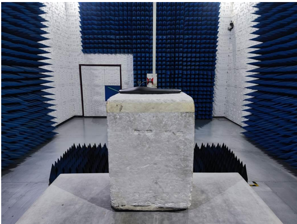
RADIATED EMISSION TEST SETUP ABOVE 1GHZ
