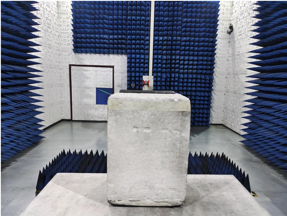
RADIATED EMISSION TEST SETUP ABOVE 1GHZ
