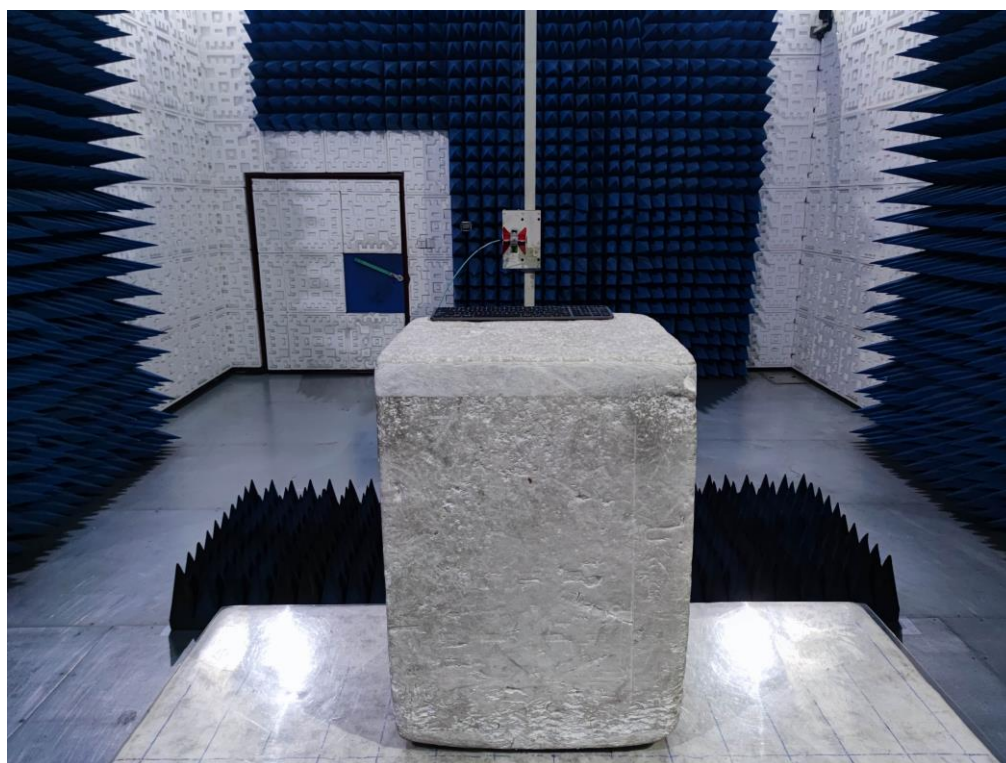
RADIATED EMISSION TEST SETUP ABOVE 1GHz
