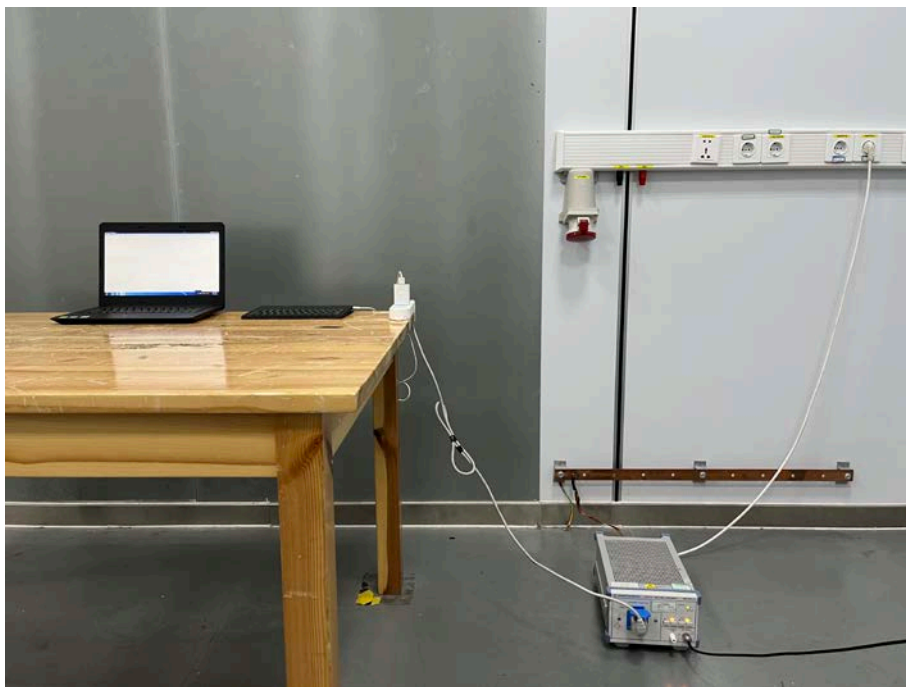
Fig. 4 Power line conducted emission setup photo
