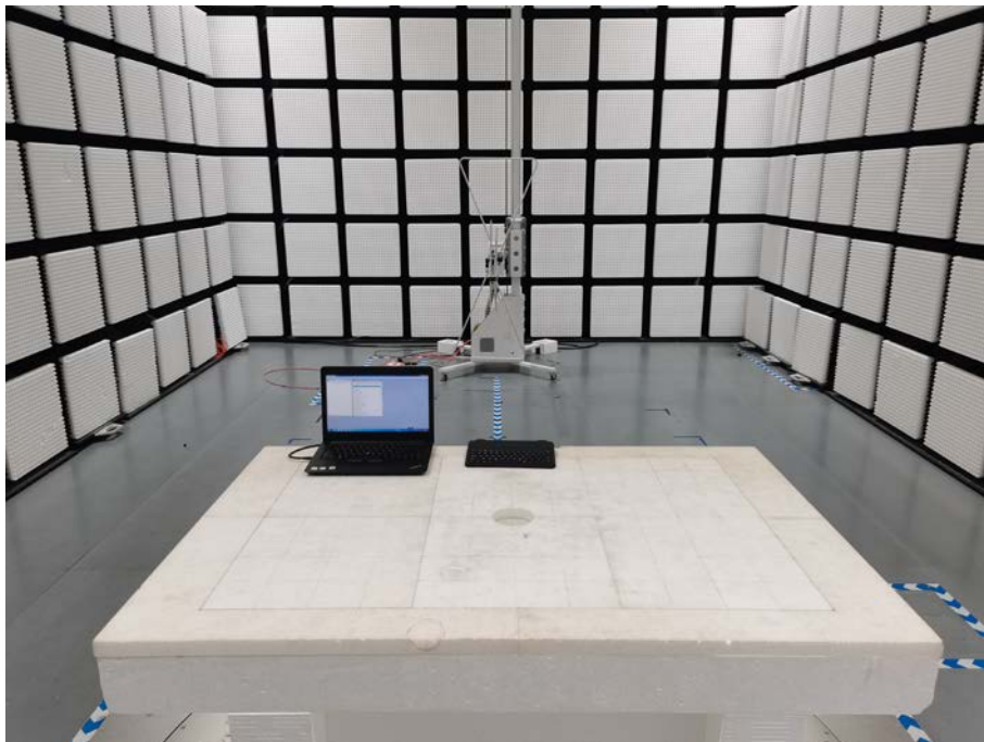
Fig. 2 Radiated emission setup photo(30MHz-1GHz)
