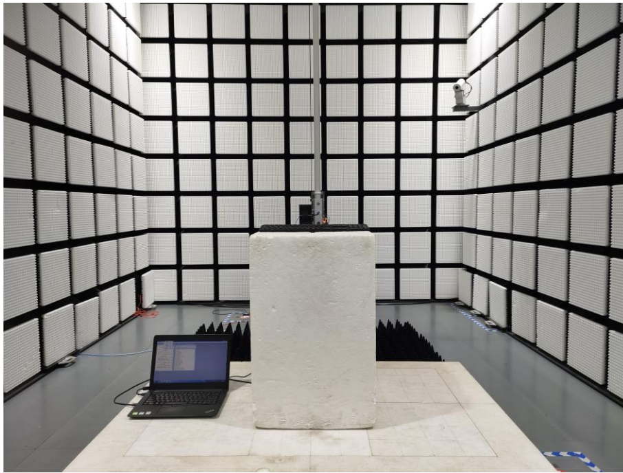
Fig. 3 Radiated emission setup photo(Above 1GHz)
