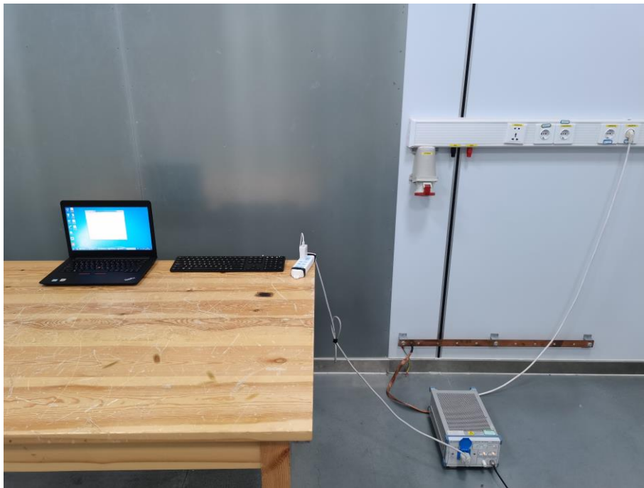
Fig. 4 Power line conducted emission setup photo
