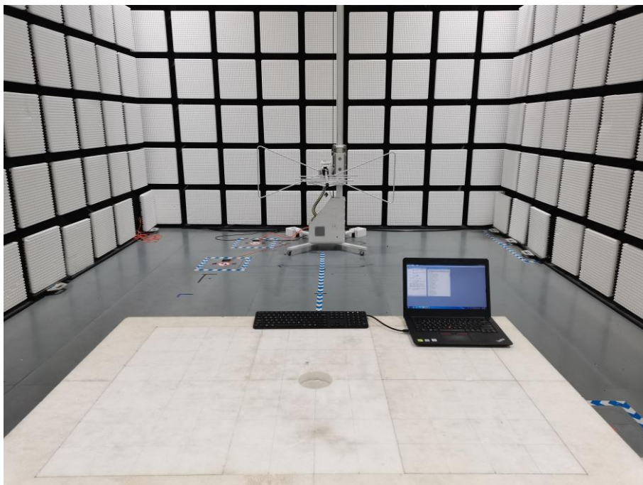
Fig. 2 Radiated emission setup photo(30MHz-1GHz)
