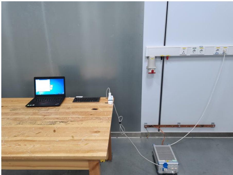
Fig. 4 Power line conducted emission setup photo
