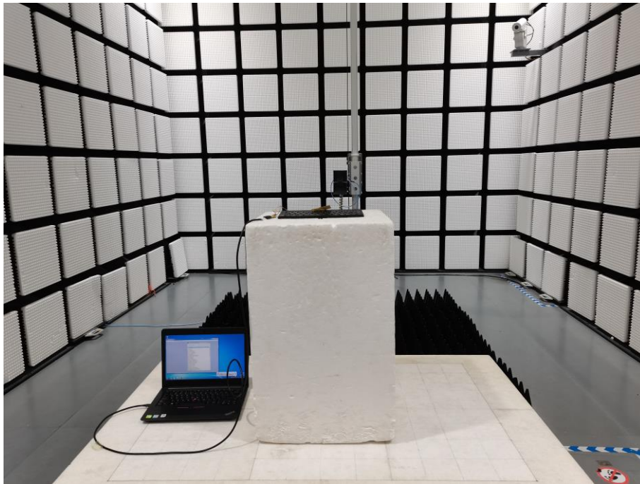
Fig. 3 Radiated emission setup photo(Above 1GHz)
