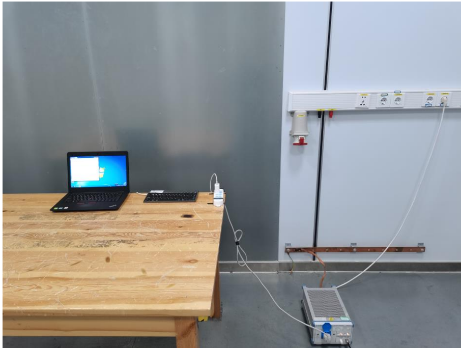
Fig. 4 Power line conducted emission setup photo
