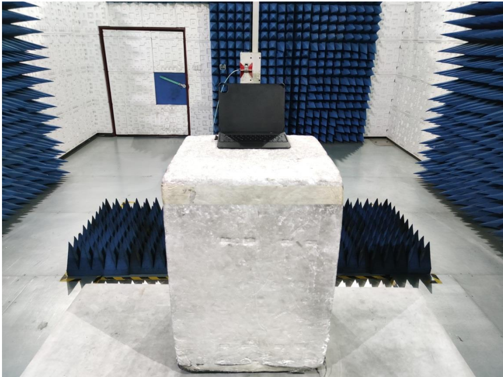
RADIATED EMISSION TEST SETUP ABOVE 1GHz
