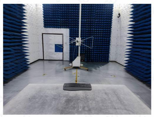
RADIATED EMISSION TEST SETUP ABOVE 1GHz
