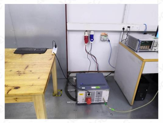
RF CONDUCTED TEST SETUP
