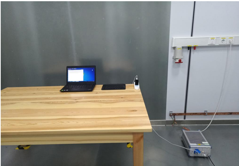
Fig. 4 Power line conducted emission setup photo
