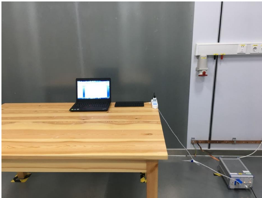
Fig. 4 Power line conducted emission setup photo
