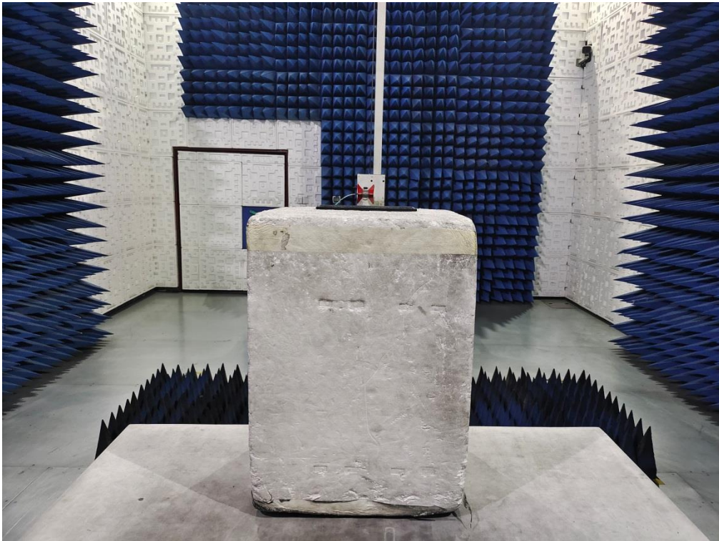
RADIATED EMISSION TEST SETUP ABOVE 1GHZ
