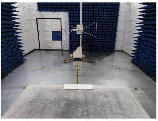
RADIATED EMISSION TEST SETUP ABOVE 1GHz
