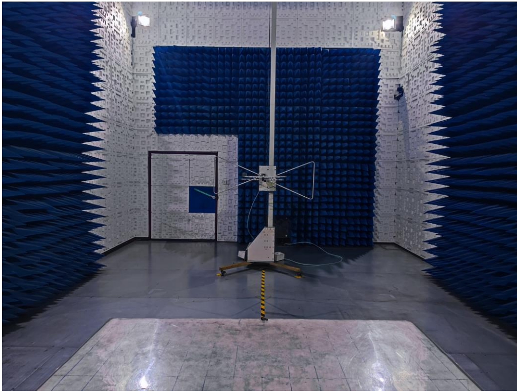
RADIATED EMISSION TEST SETUP ABOVE 1GHz
