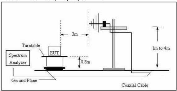
(C) Radiated Emission Test-Up Frequency Above 1GHz
