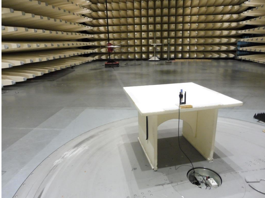
Photo 7: EUT at the semi-anechoic chamber
