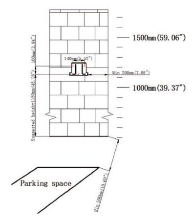
Step 2: Hang the charger on the mounting back plate as shown below:
