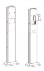
Step 2: Hang the whole charger on the installation plate, as shown in the figure below:
