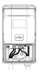
Step 7: Reinstall the wiring cover as shown below:
