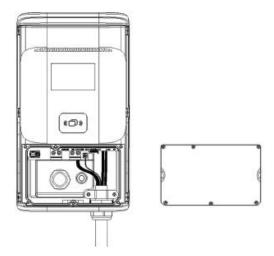
Step 6: Access the AC input power line as shown below:
