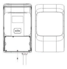
Step 5; Remove the wiring cover as shown below:
