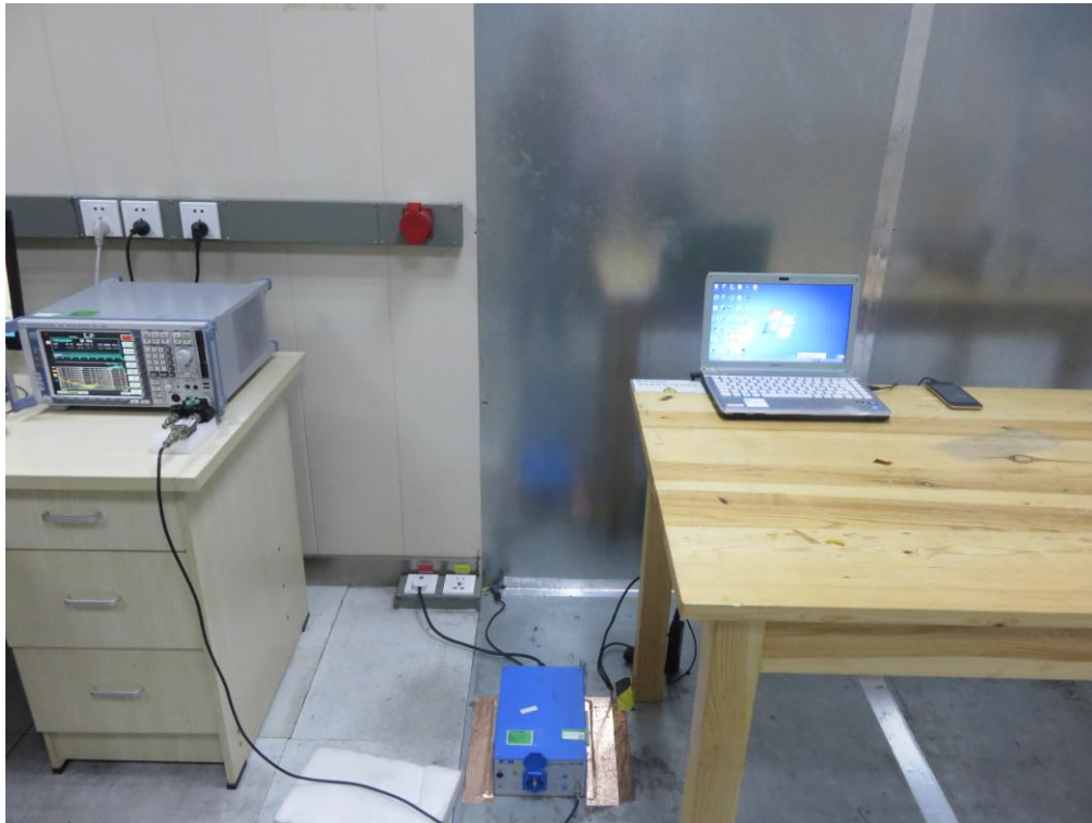
FCC RADIATED EMISSION TEST SETUP
