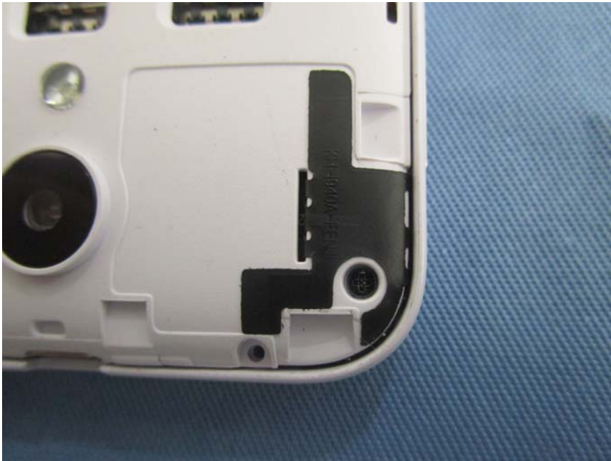
EUT – LTE RX Antenna View
