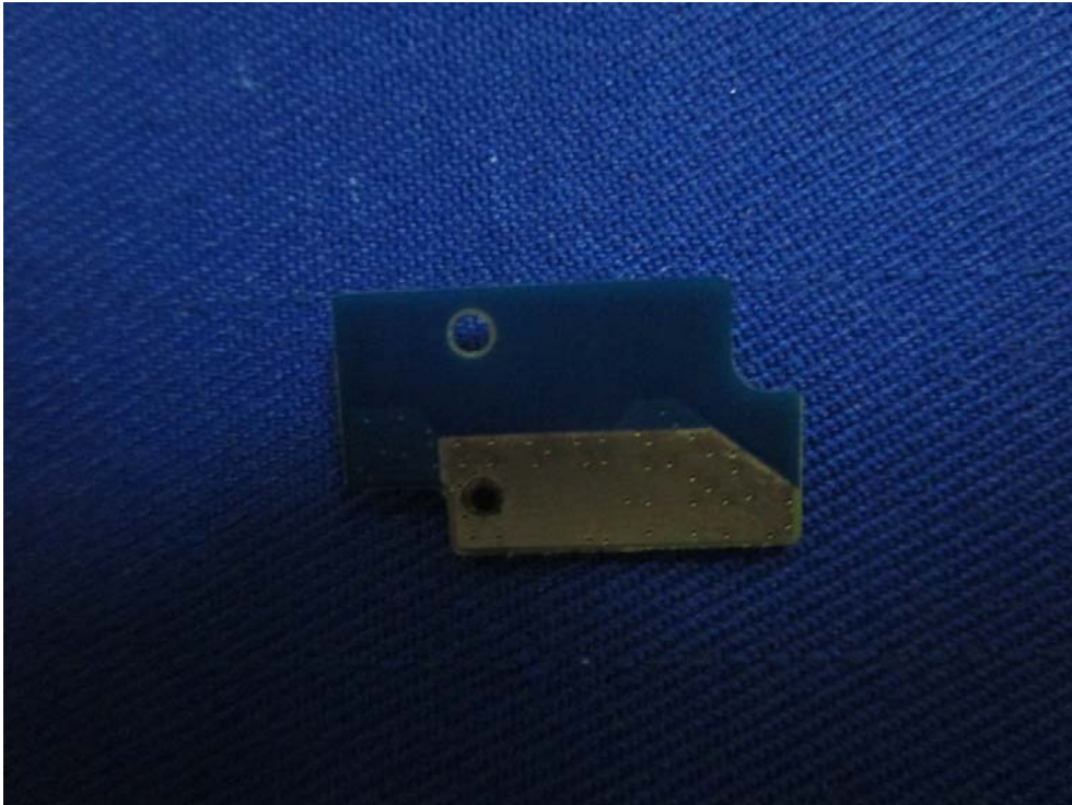
EUT –ANT PCB Back View
