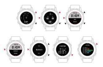
In the movement, press BACK key to pause the view amd return to view the movement data, press BACK in the data view to return to the pause menu view again.
