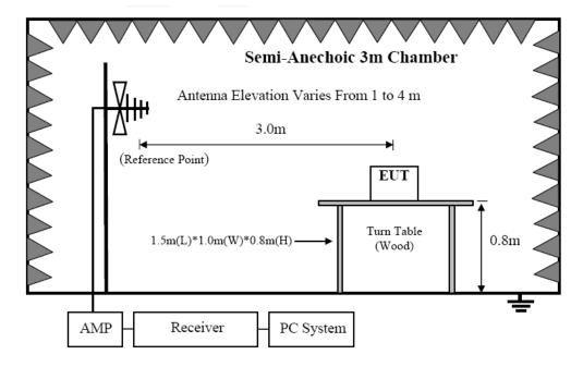
8.2.3 In 3m Anechoic Chamber Test Setup Diagram for frequency above 1GHz
