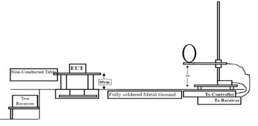
8.2.2 In 3m Anechoic Chamber Test Setup Diagram for 30MHz to 1GHz
