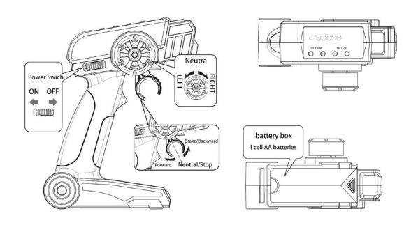
WARNING: BATTERIES ARE SUITABLE FOR 4 ALKALINE BATTERIES. ENSURE THAT THE POSITIVE AND NEGATIVE POLES OF THE BATTERIES ARE INSTALLED CORRECTLY. THE INCORRECT POLARITY OF THE BATTERIES WILL CAUSE DAMAGE TO THE REMOTE CONTROL. LED INDICATES TRANSMITTER BATTERY VOLTAGE STATUS, WHEN ONLY ONE LED LAMP IS ON, THE BATTERY VOLTAGE IS LOW, PLEASE REPLACE THE BATTERY IN TIME!
