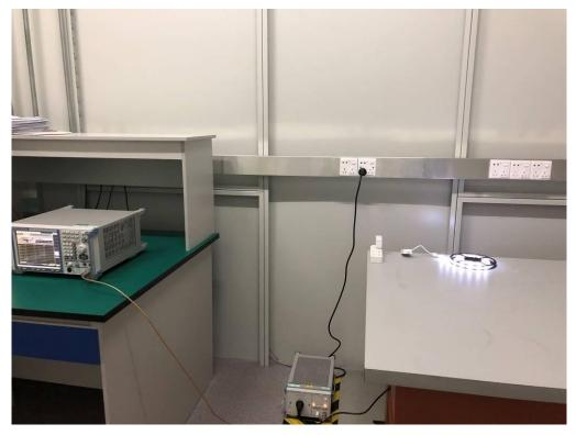
FCC RADIATED EMISSION TEST SETUP
