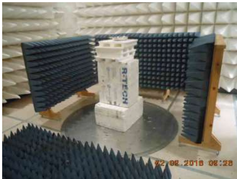
Above 1GHz Cone placement
