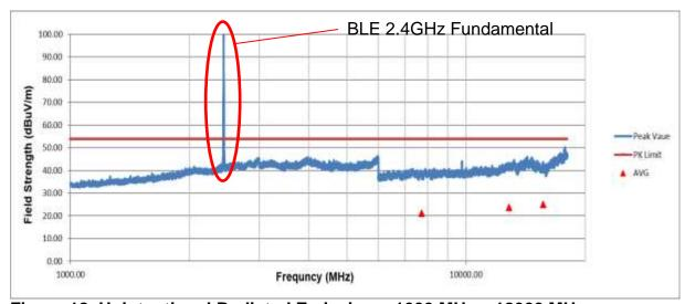
Figure 18. Unintentional Radiated Emissions, 1000 MHz – 18000 MHz (Horizontal)
