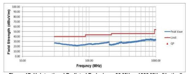
Figure 17. Unintentional Radiated Emissions, 30 MHz – 1000 MHz (Vertical)
