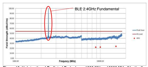
Figure 19. Unintentional Radiated Emissions, 1000 MHz – 18000 MHz (Vertical)
