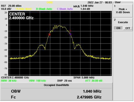
Figure 12. 99% Occupied Bandwidth High Channel PHY1
