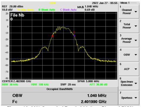
Figure 10. 99% Occupied Bandwidth Low Channel PHY1
