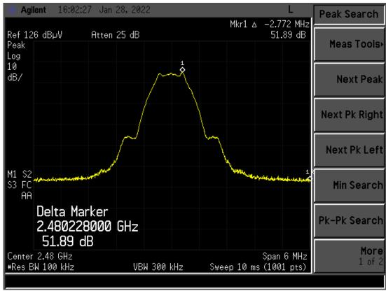
Figure 6. Band Edge Compliance, High Channel PHY1 Delta, Peak
