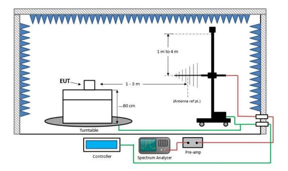
Figure 1. Block Diagram of Test Configuration
