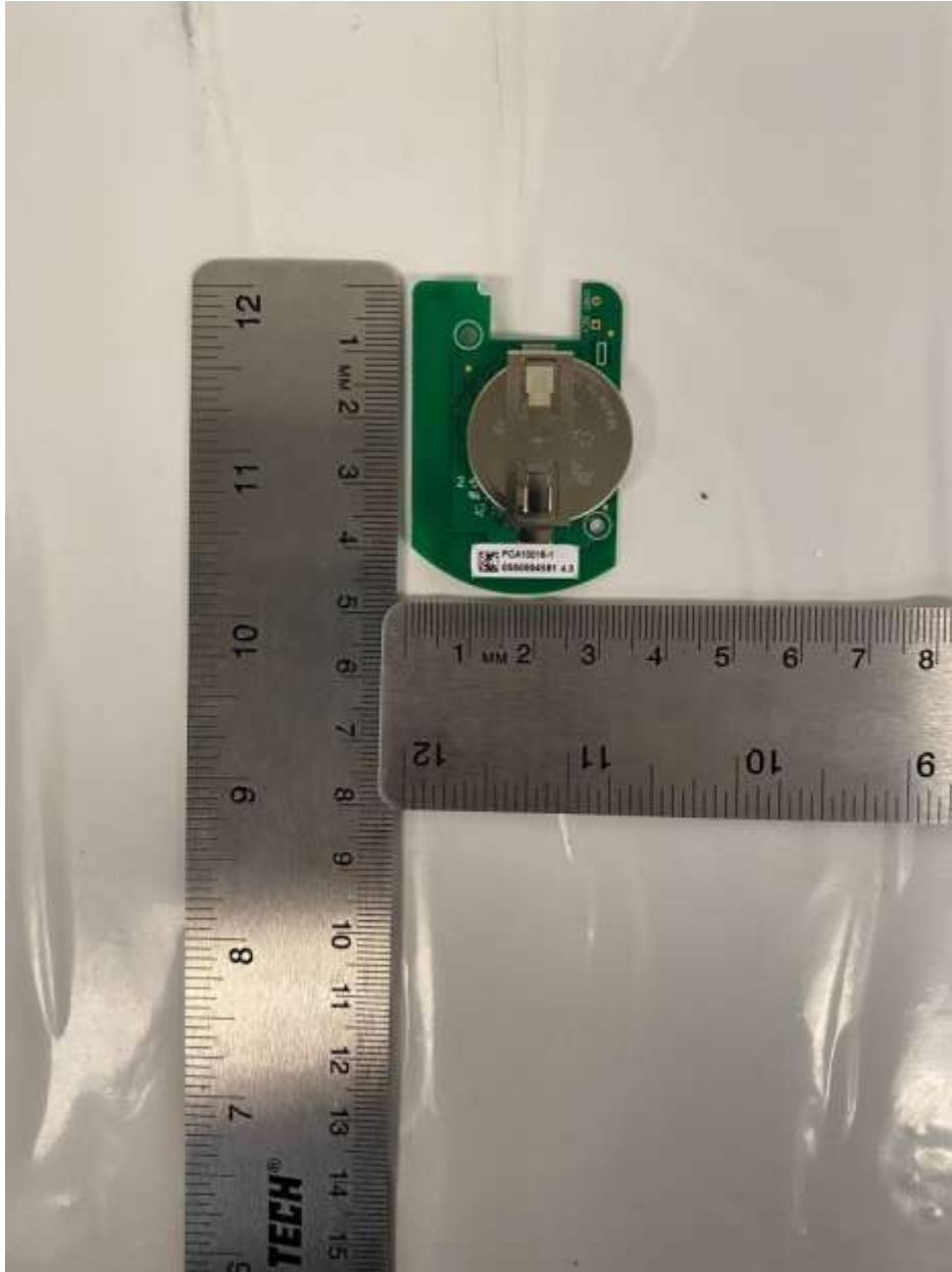
Figure 3. PCB Side 2 (with Battery)
