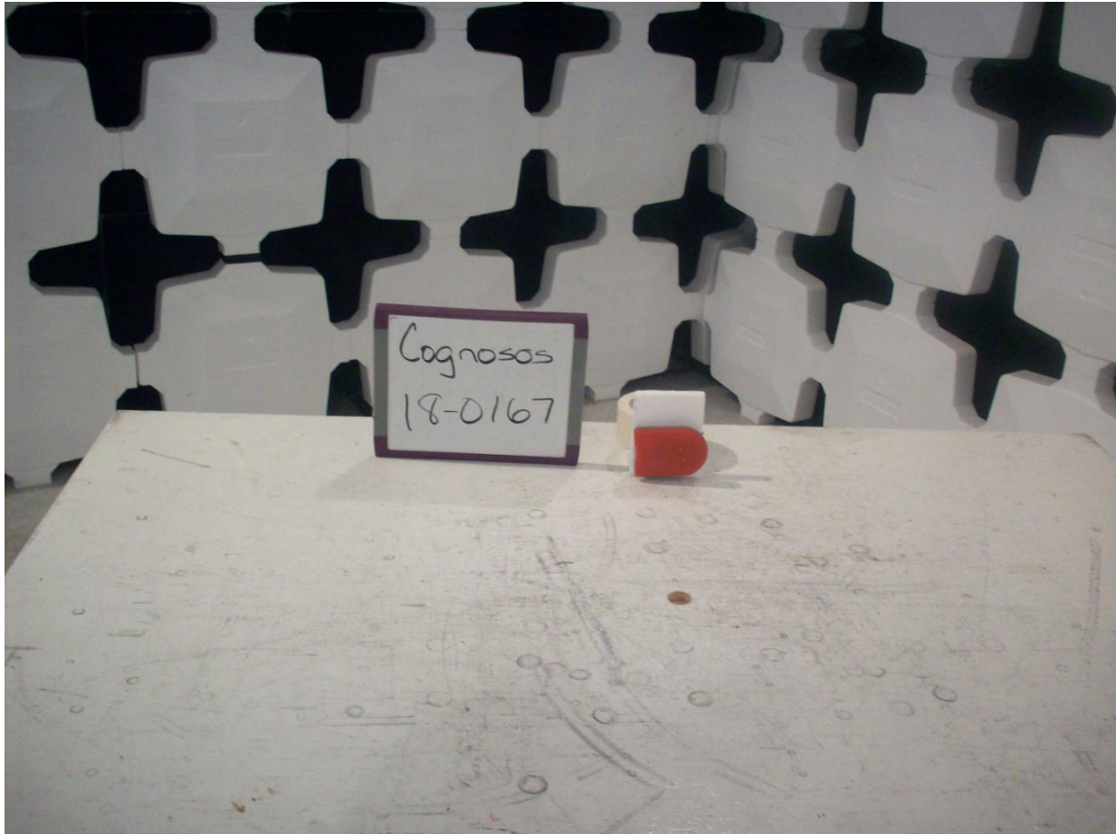
Figure 1. EUT Radiated Emissions Test Setup
