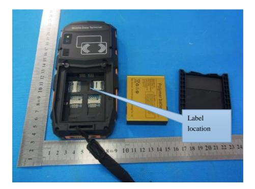
Size:20\*15mm M/N: C5000 FCC ID: 2AKFLC5000 This device complies with part 15 of the FCC Rules. Operation is subject to the condition that this device does not cause harmful interference. MOVIC FON
