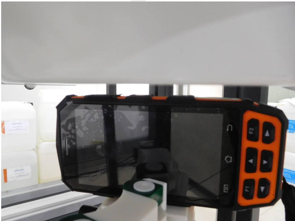
Body right side(separation distance is 5mm)
