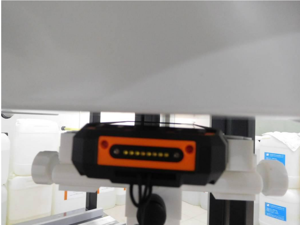
Body Front side(separation distance is 5mm)
