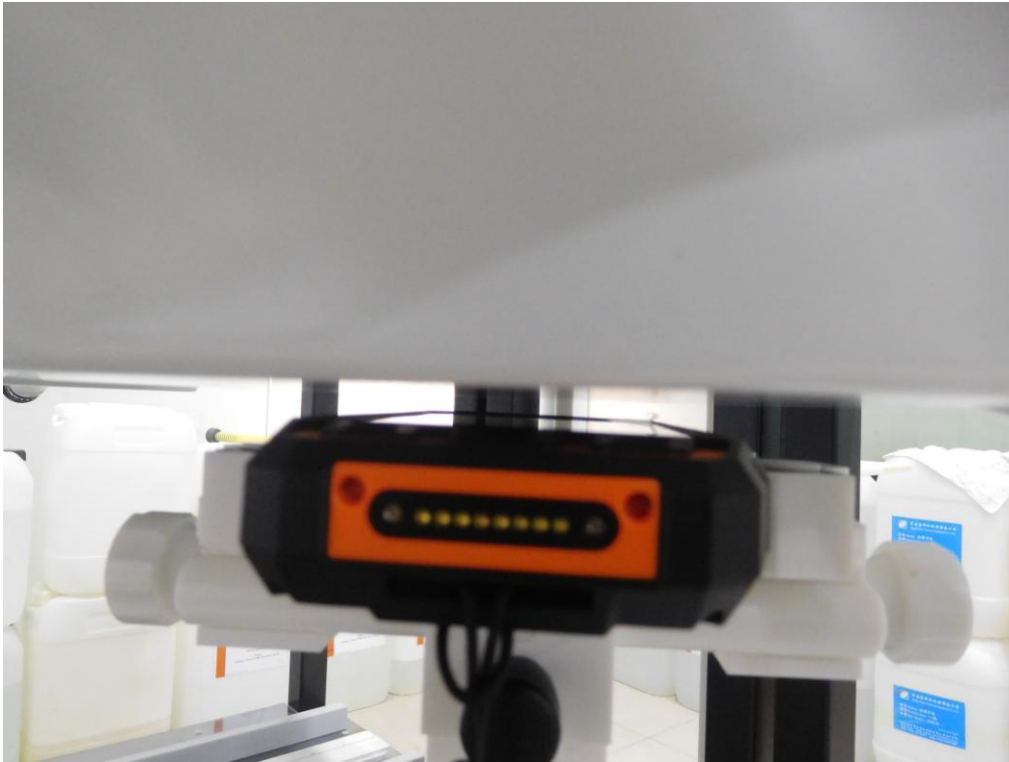
Body Front side(separation distance is 5mm)
