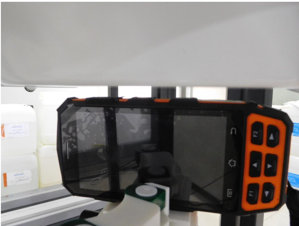
Body right side(separation distance is 5mm)
