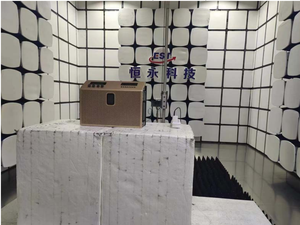
Radiated Test (Above 1GHz)
