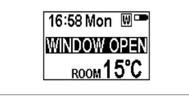
2b.45 After indoor temperature rise or manual intervention (by operating remote control), it will return to normal working state.
