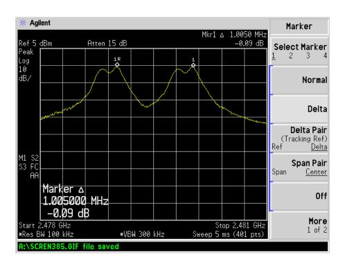
For 8DPSK mode Channel Spacing (Low CH=1MHz)
