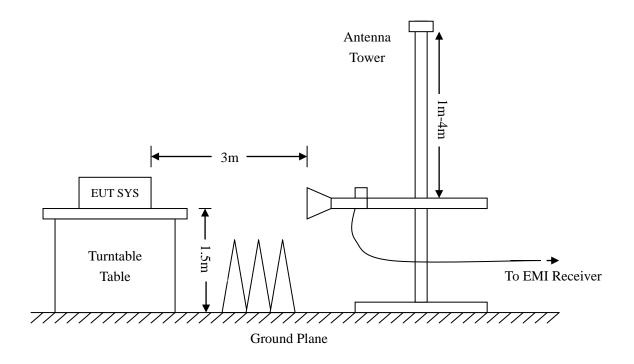
Frequency :9kHz-30MHz Frequency :30MHz-1GHz Frequency :Above 1GHz RBW=10KHz, RBW=120KHz, RBW=1MHz,
