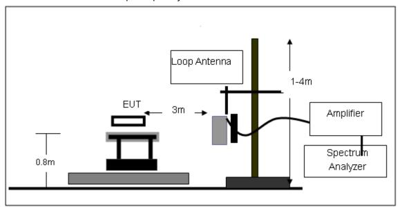
(B) Radiated Emission Test-Up Frequency 30MHz~1GHz
