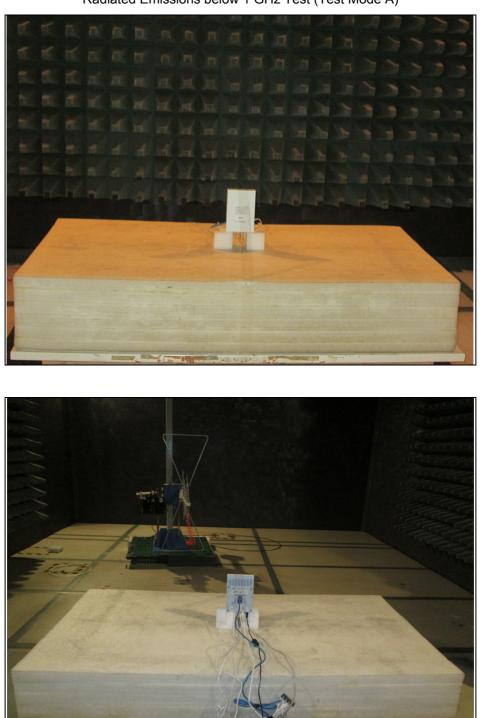
Radiated Emissions below 1 GHz Test (Test Mode A)
