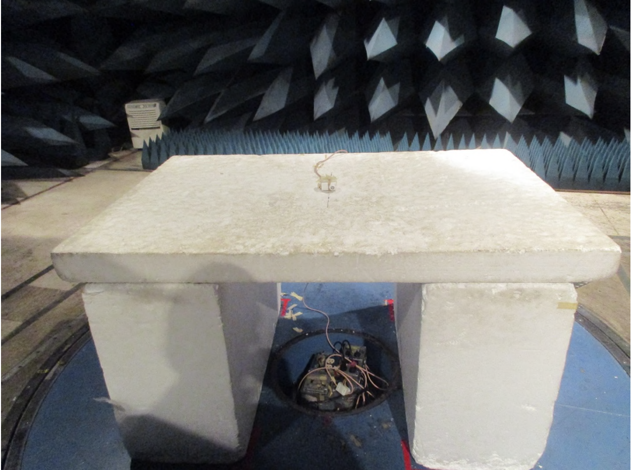
Figure 7: Radiated Emissions – Front View - Below 1 GHz – EUT on Side
