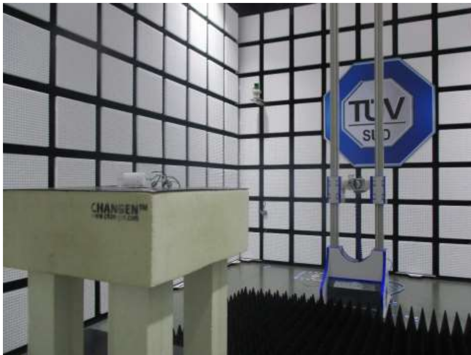
Radiated Emission test 18-25GHz
