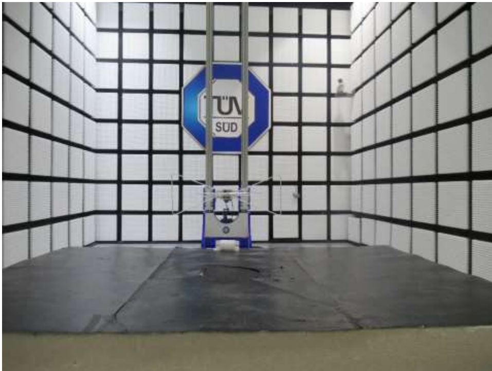
Radiated Emission test of 30MHz-1GHz
