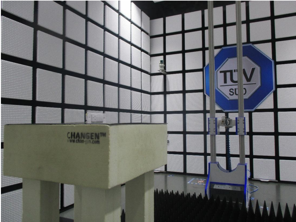
Radiated Emission test 18-25GHz
