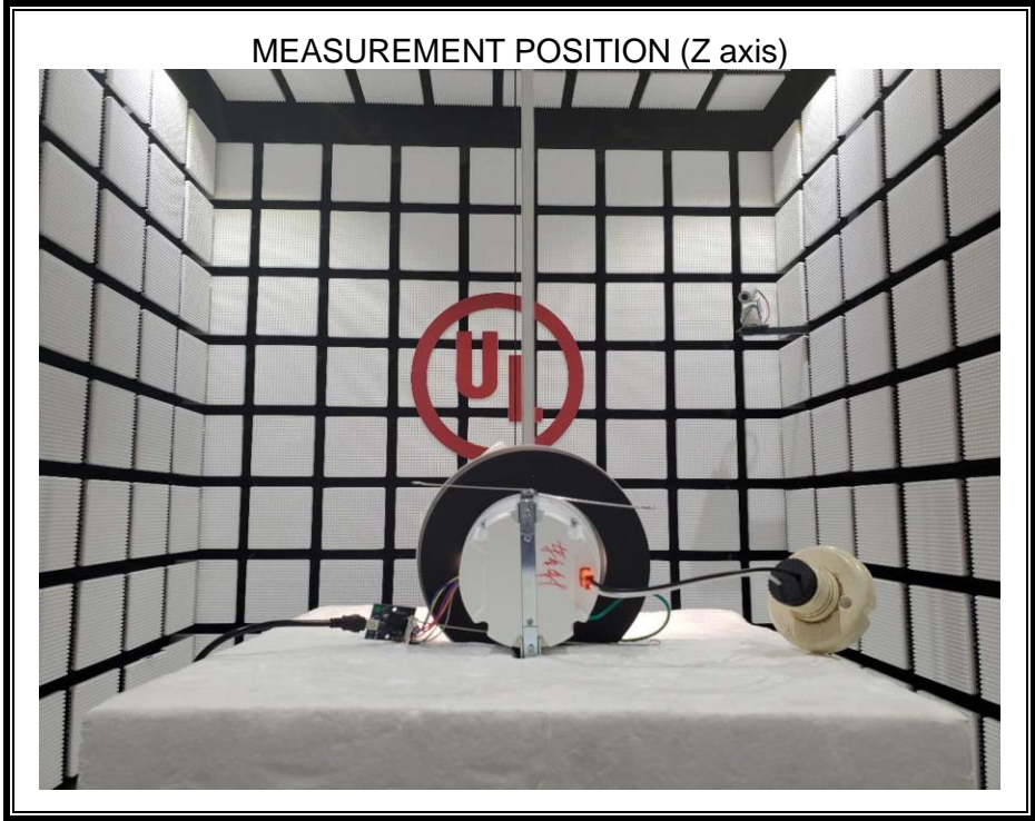
RADIATED RF MEASUREMENT SETUP (30MHz~1GHz)
