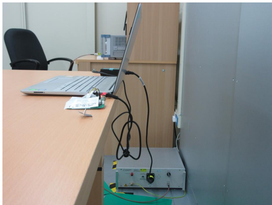
Photograph 8: Set-up for AC Mains (Back View)
