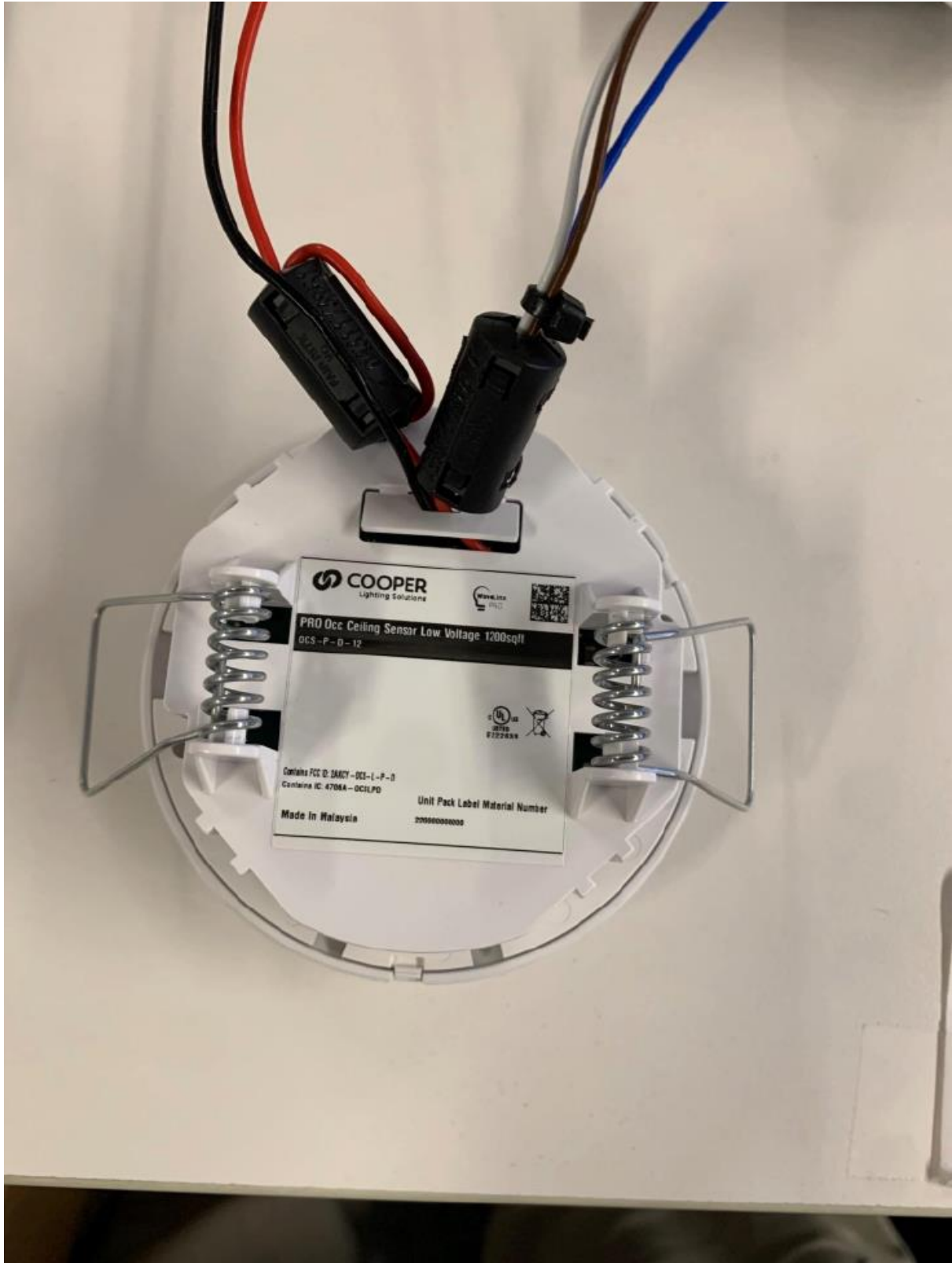
Label Location – Low Voltage
