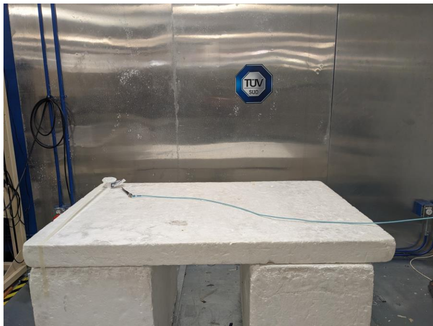
Figure:11– Test Set up – Power Line Conducted Emissions
