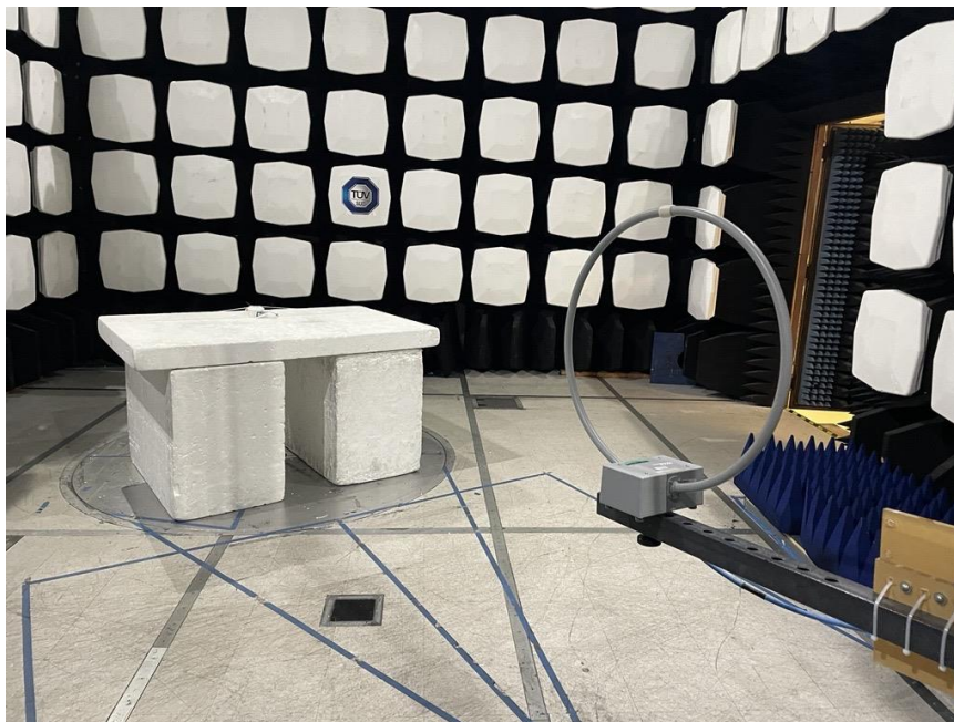
Figure:1 – Test Set up – Front View of the EUT - Radiated Emissions <30 MHz
