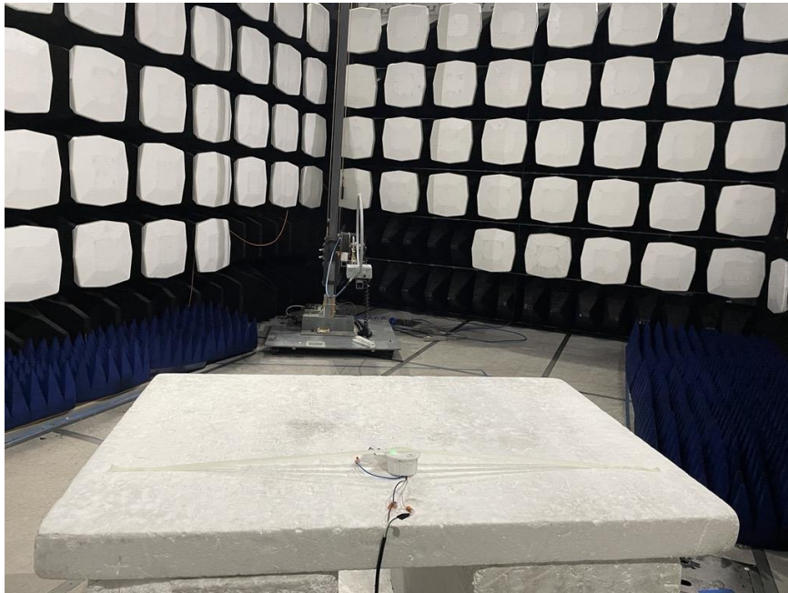
Figure:2 – Test Set up – Rear View of the EUT- Radiated Emissions <30 MHz
