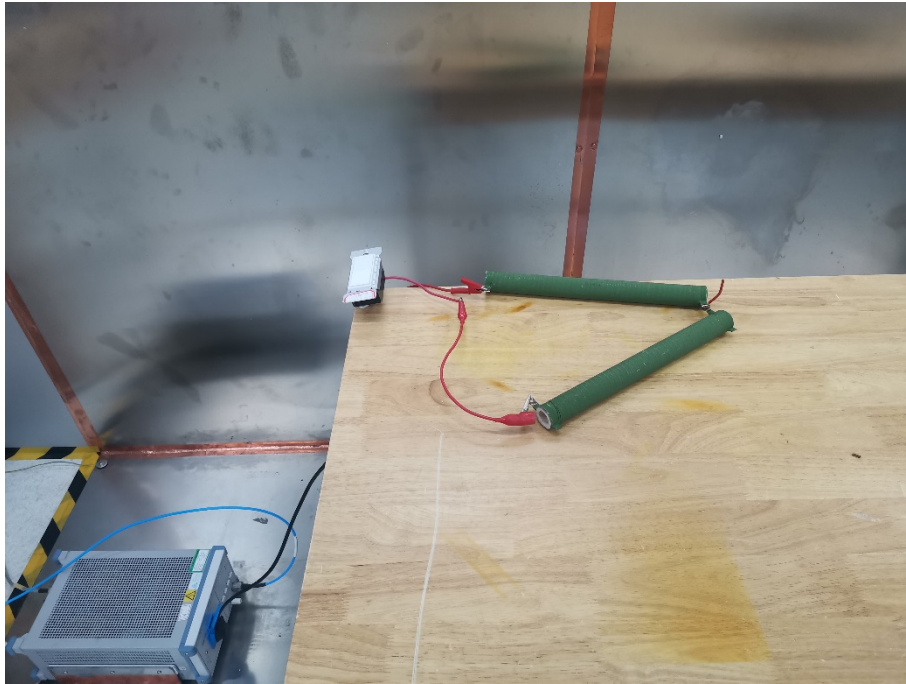
Photograph 3: Set-up for Conducted Emissions ON AC mains
