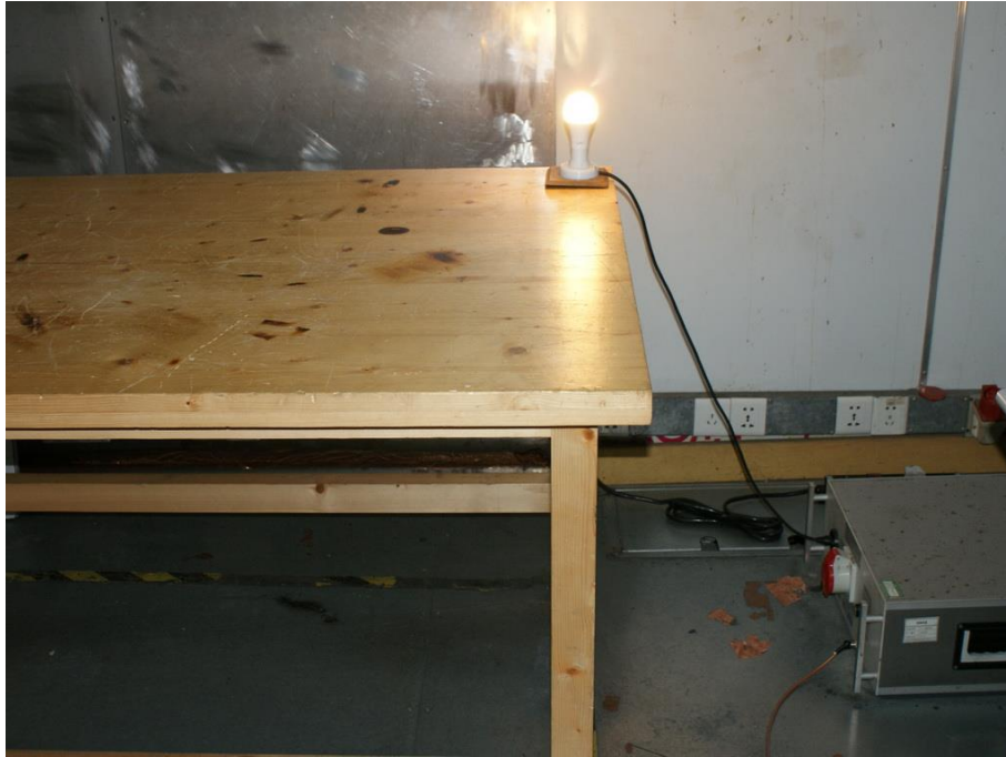
Photograph 1: Set-up for Conducted Emission on AC Mains
