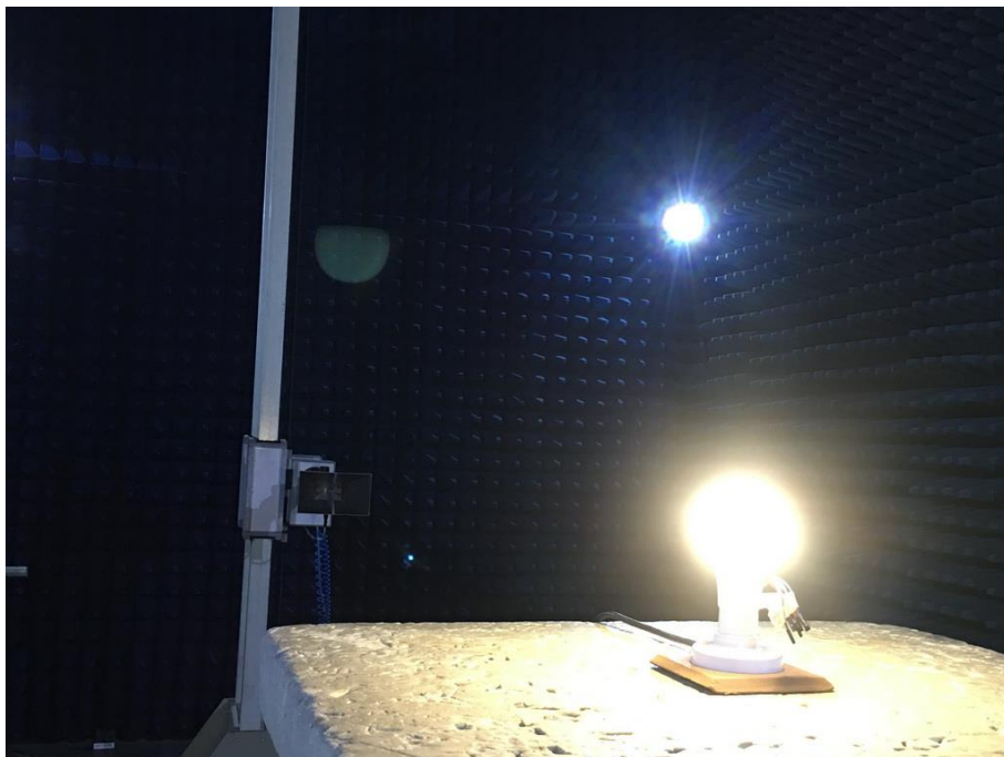
Photograph 6: Set-up for Radiated Spurious Emission, 1GHz - 18GHz
