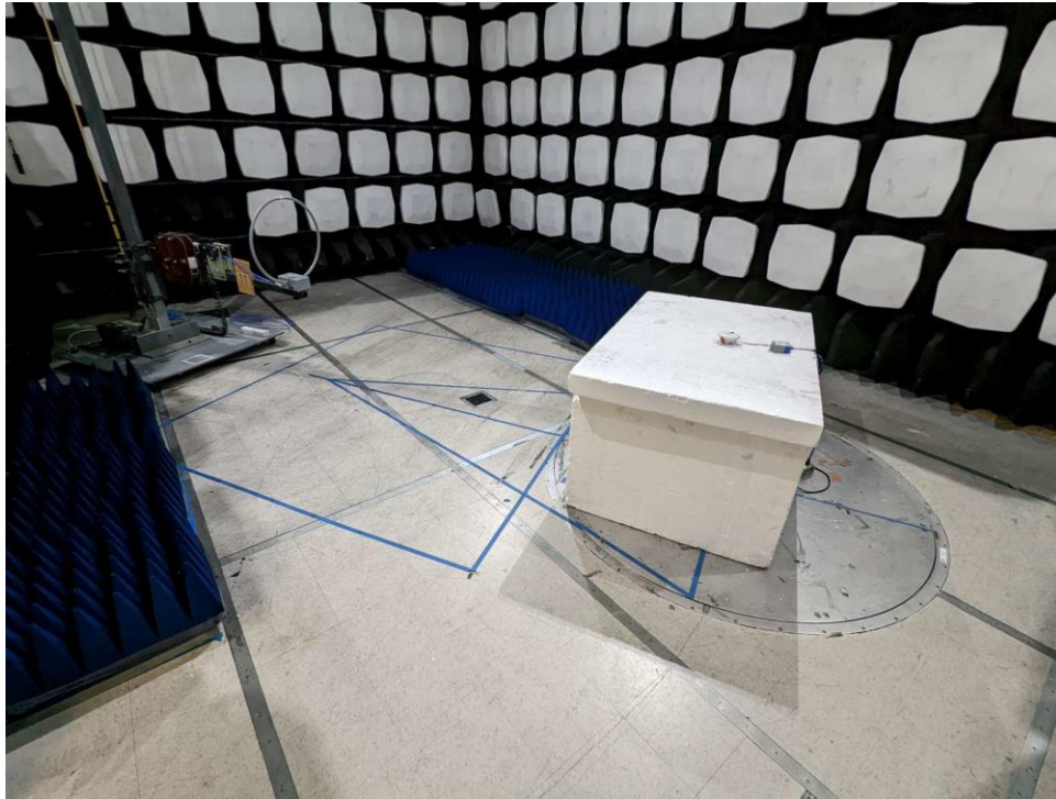
Figure 1: Test Setup – Radiated Emissions <30MHz
