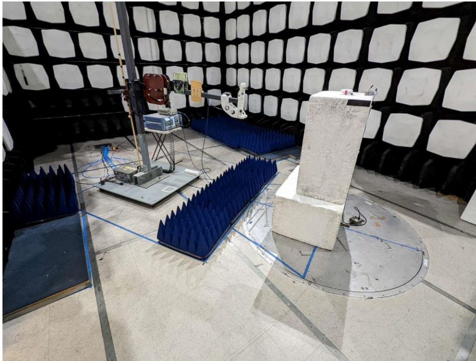
Figure 5: Test Setup – Radiated Emissions >18GHz
