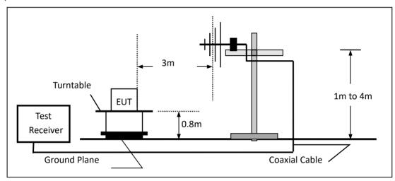
(c) For radiated emissions above 1000MHz
